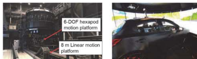
Fig.5 Driving simulator used for the experimental test
